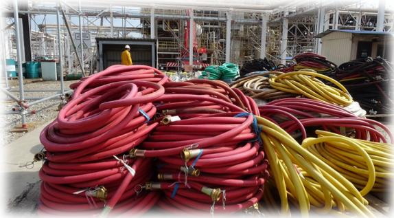
Hose assemblies in manufacturing or processing plants can sometimes be the source of equipment malfunction, dangerous product spills, or serious personnel injury. With today's increasing need for faster and quicker fluid transfers, the demands being placed on hose assemblies are greater than ever due to increased working temperatures and pressures, that can easily diminish their containing power.
